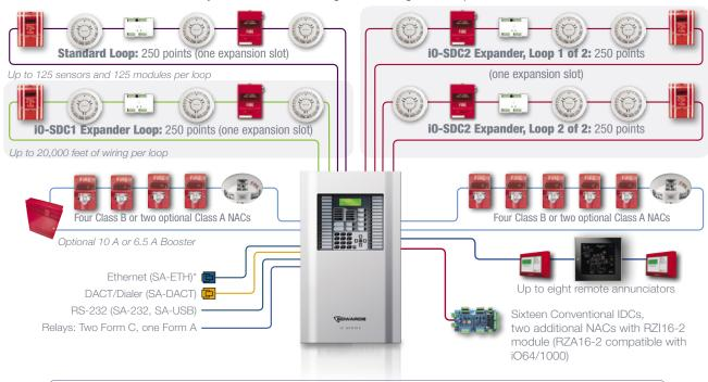
Each iO1000 panel supports 1,000 addressable devices, has room for up to two Signature loop controller cards with expansion capacity in any combination of single or dual 250-device loops. iO1000 addressable loops support 125 detectors and 125 modules.
